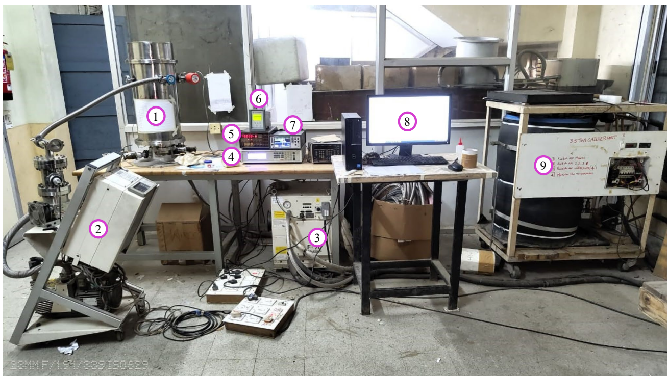
Fig. 4 Experimental setup (1) Cryocooler (2) Turbomolecular pump (3) Compressor (4) Temperature controller (5) Constant current source (6) Pressure gauge (7) DAQ (Data Acquisition system) (8) PC {LabVIEW program} (9) Chiller unit
