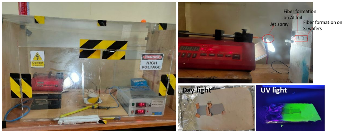
Figure S5. Electrospinning set up and nanofiber deposition on Si wafer and Al foil (up right), deposited fibers on Al foil and Si wafer under UV light and day light (below right).
