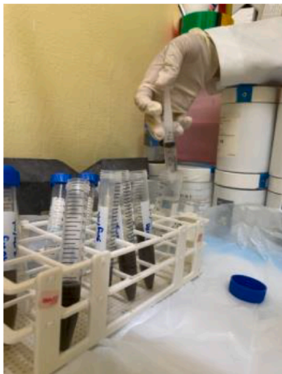
Fig. 1. Preparation of 1.0, 2.0, 3.0, 4.0 and 5.0 mg/mL concentrations of adsorbents using syringe.
