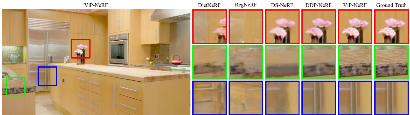
Figure 7: Qualitative examples on RealEstate-10K dataset with two input views. We observe sharp predictions by ViP-NeRF while predictions by other models suffer from blur and other artifacts. In particular, DDP-NeRF predictions contain blurred flowers (first row) and blurred tiles (second row).
