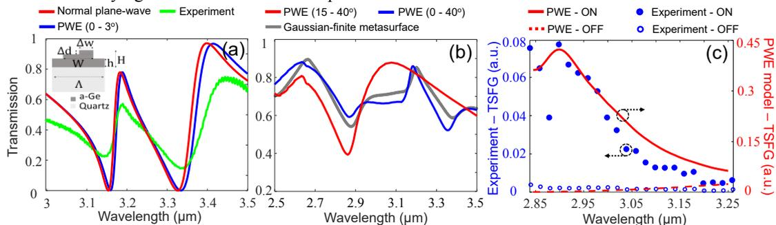
Fig. 1: (a) Experimental and simulated transmission spectra under normal incidence plane-wave and PWE model (inset shows metasurface unit-cell). (b) Transmission spectra calculated with PWE for 15-40°, 0-40° and gaussian excitation of finite metasurface. (c) Experimental and simulated TSFG spectrum shown on- and off- the metasurface.
