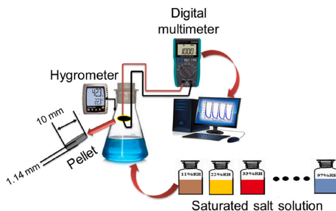
Fig. 1. Schematic of the humidity sensor experimental setup.
