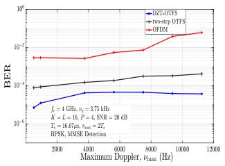
Fig. 5: BER performance of DZT-OTFS, two-step OTFS, and OFDM as a function of maximum Doppler,  $\nu_{\text{max}}$ .
