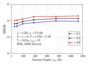
Fig. 6: Effect of RC pulse roll-off factor,  $\gamma$ , on BER vs  $\nu_{\rm max}$  performance.
