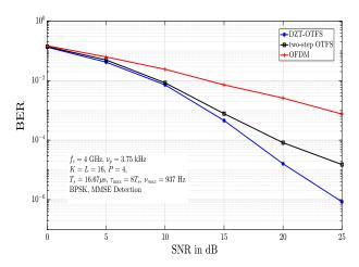
Fig. 4: BER performance of DZT-OTFS, two-step OTFS, and OFDM as a function of SNR.
