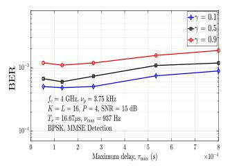
Fig. 7: Effect of RC pulse roll-off factor,  $\gamma$ , on BER vs  $\tau_{\rm max}$  performance.
