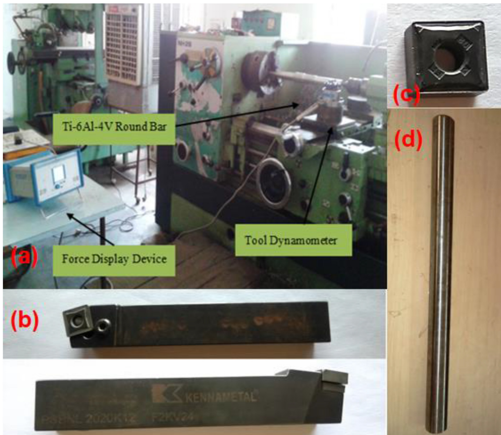
Fig. 2 – (a) Experimental setup; (b) Tool holder; (c) KC5010 cutting insert; (d) Ti-6Al-4V round bar [14].
