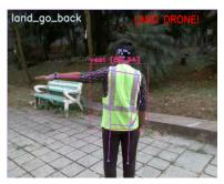
(c) VIP gesturing for drone to land (Drone camera view)
