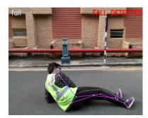
(d) VIP in safe upright position (Drone camera view) (e) VIP kneeling upon a simulated injury (Drone cam view) (f) VIP after a simulated fall (Drone camera view)
