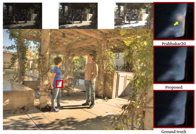
Fig. 6. A qualitative example from Kalantari17 dataset [18]. The red zoomed box highlight the artifact introduced by the Prabhakar20 method on saturated dynamic regions. Comparatively, the proposed method can generate plausible textures, even in saturated areas. Image best viewed electronically.
