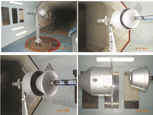
Figure 3. Crew Model separation studies in a wind tunnel.
