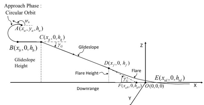
Fig. 1. Autonomous landing Phases of an Unmanned Aerial Vehicle
