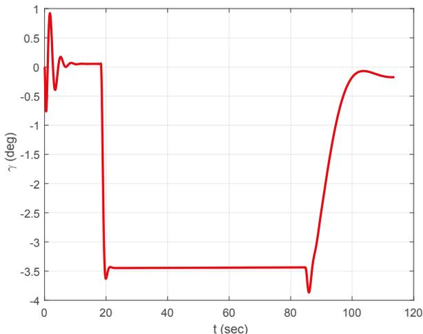
Fig. 9. Flight path angle profile of autoland UAV
