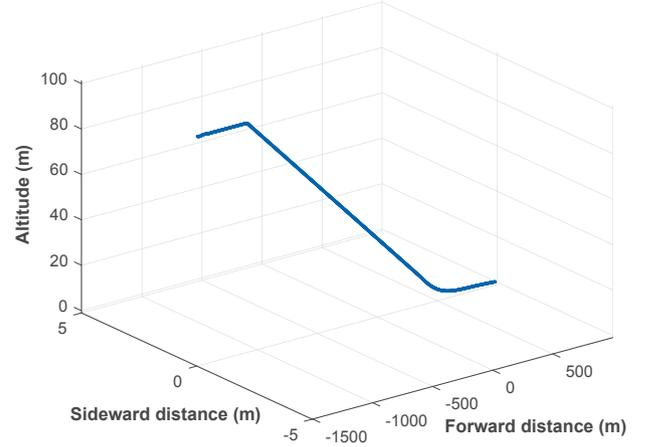
Fig. 5. Autonomous landing trajectory of UAV
