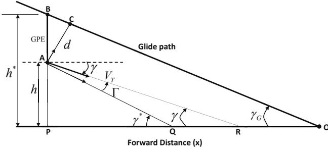
Fig. 2. Glideslope Altitude and Gamma Error Computation
