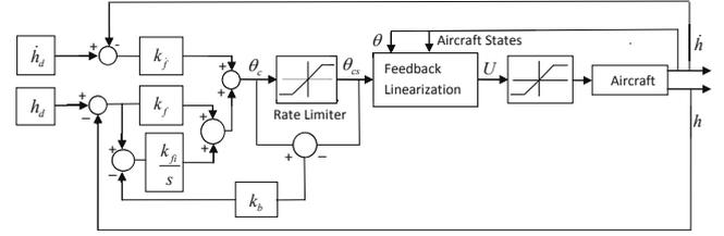
Fig. 4. Flare autopilot block diagram with Anti Windup
