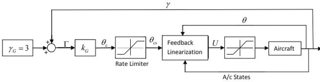
Fig. 3. Glideslope autopilot block diagram
