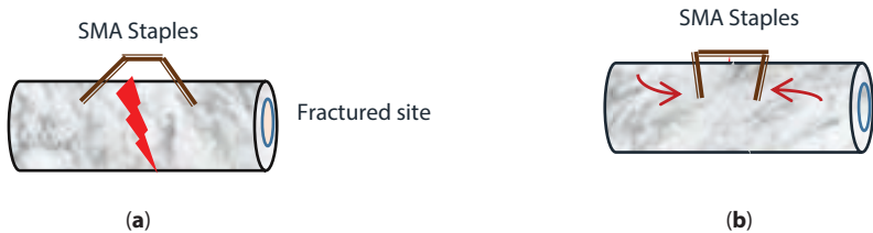
Figure 2.7 Medical SMA staple: (a) un-actuated-martensite state; (b) actuated-austenite state.
