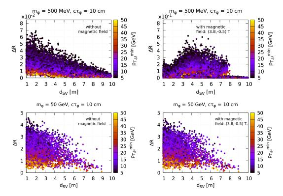
FIG. 7. Variation of the  $\Delta R$  values between the muons coming from the decay of the boosted LLP (mediator particle  $\phi$ ) as a function of the distance between the secondary vertex and the IP,  $d_{SV}$ , with (right panels) and without (left panes) the 3.8 T solenoidal magnetic field. The color bar shows the minimum  $p_T$  from the muon pair.
