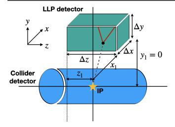
FIG. 40. Illustration of the parameters denoting position and size of the decay volumes for DELIGHT detector, a box-type LLP detector near the IP of the 100 TeV collider.
