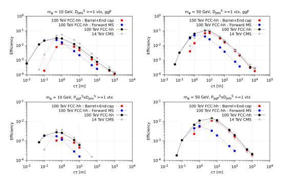
FIG. 35. Comparison of the efficiencies as a function of decay lengths, as obtained from the  $D_{jets}^S \ge 1$  vtx (top) and  $P_{ggF}^S \times D_{jets}^S \ge 1$  vtx (bottom) sets of cuts between the CMS MS at 14 TeV and FCC-hh MS at 100 TeV, when a mediator of mass 10 GeV (left) and 50 GeV (right) decays to a pair of b quarks. For the FCC-hh detector, we also show the efficiencies for the barrel and end cap MS and the forward MS separately.
