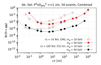
FIG. 36. Comparison of the projected upper limits on the branching fraction,  ${\rm Br}(h\to\phi\phi)$ , for 50 observed decays of long-lived mediator particles into a pair of b quarks within the CMS and the FCC-hh MS for the  $P^S\times D^S_{jets}\geq 1$  vtx set of cuts. The shown limits are obtained by combining the ggF, VBF, and VH modes for the Higgs boson production.
