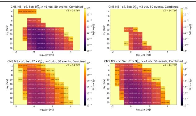
FIG. 21. Projected upper limits on  $Br(h \to \phi \phi)$  for 50 observed decays of long-lived mediator particles decaying into a pair of c quarks within the CMS MS for four sets of cuts explained in the text. The shown limits are obtained by combining the ggF, VBF, and VH modes of the Higgs boson production at the 14 TeV HL-LHC experiment (3000 fb<sup>-1</sup>).
