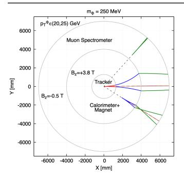
FIG. 6. Transverse projection of the propagation of a muon pair in the magnetic field of the CMS detector, where the pair is assumed to be from the decay of the LLP ( $m_{\phi} = 250$  MeV) that is pair produced from the Higgs boson decay. See text for more details.
