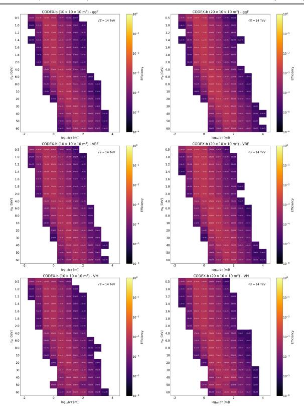
FIG. 43. Efficiency maps for decays of long-lived mediator particles within the CODEX-b detector for the ggF (top), VBF (center), and VH (bottom) production of the Higgs boson.
