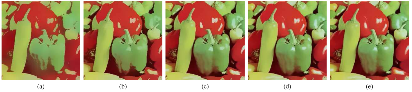
Fig. 10. Bilateral filtering of Peppers for different values of K ( \sigma_s = 10 and \sigma_r = 40 ). Notice how the accuracy improves with K . (a) K = 2 (15 ms, 22 dB). (b) K = 4 (28 ms, 29 dB). (c) K = 8 (52 ms, 37 dB). (d) K = 16 (100 ms, 44 dB). (e) Brute-force.
