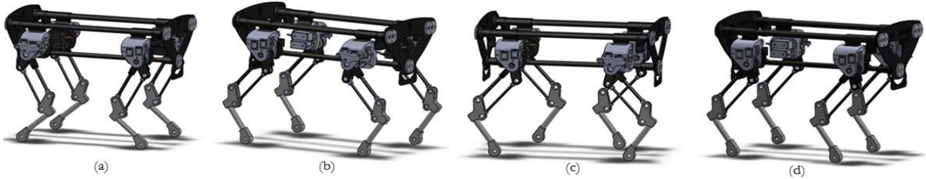
Figure 3. Modular configurations of Stoch: (a) X configuration, (b) O configuration, (c) XO configuration, (d) natural quadruped configuration.
