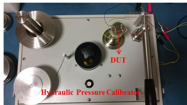
Fig. 5 Pressure sensor mounted on hydraulic pressure calibrator
