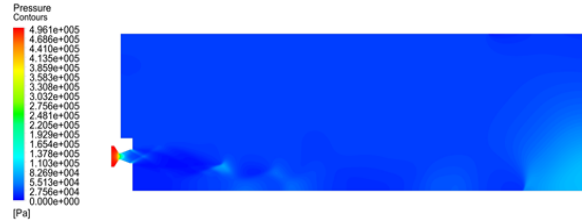
Fig. 16. Pressure contours for launch pad and guide stand case
