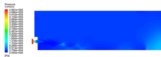
Fig. 12. Pressure contours for with launch pad and guide stand case
