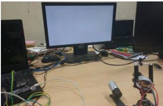
Figure 8. Setup of Laser Pointer for Exposure Test
