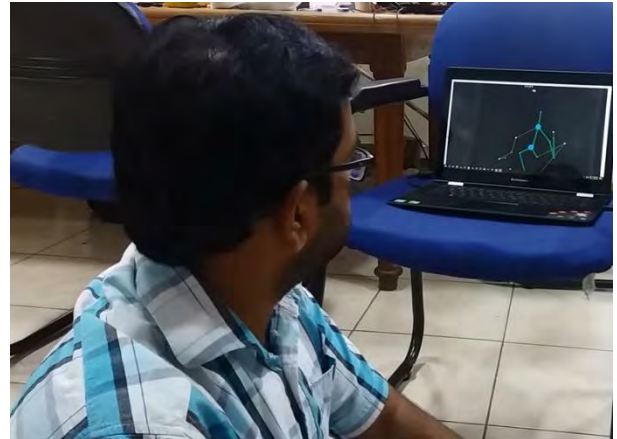
a. Torso turned less than 60°, indicated by the blue dots in the Kinect Skeleton Model
