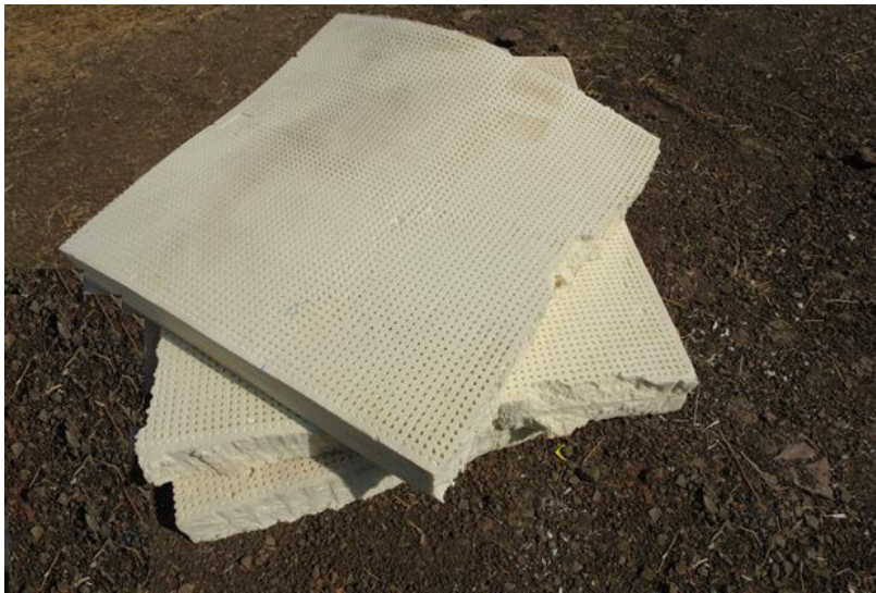
Fig. 3 Pin core natural latex polymer foam used in the experiments. Foam density 20 kg/m 3 .
