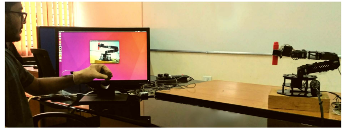
Fig. 7. Demonstration of a TCPS application using TCPSbed — a human operator wears a tactile glove and controls a remote-side robotic arm to pick and place objects.
