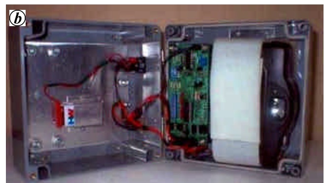
Figure 2. a , Trap developed and used for the study. b , Inside view of the camera trap.
