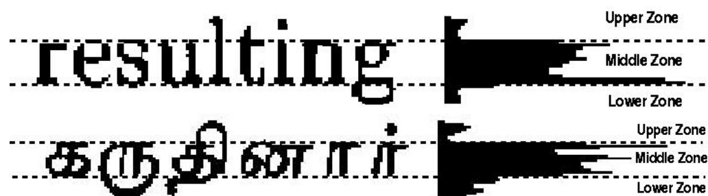
Figure 2. The three distinct zones of (a) an English word and (b) a Tamil word, and their corresponding projection profiles.
