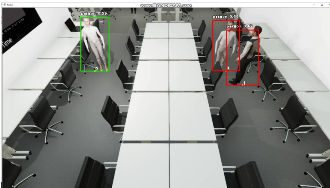
Figure 4 Humanoids detected by person detection model and annotated with bounding boxes. Here, the bounding boxes turn to red if social distancing is violated and are otherwise green.
