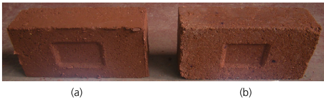
Figure 8. Comparison of the control (a) and activated (b) block specimens immediately after compaction and demoulding
