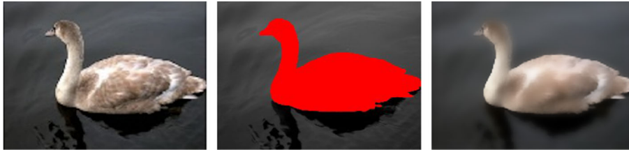
Fig. 2 Left: An image of dimensions 548 \times 402 from the Weizmann 1-object database [2]. Middle: Two labels are used to segment the pixels. The pixels belonging to the foreground are identified by the colour-code red. Right: The image on left is filtered using a bilateral filter [50]. A bilat-
