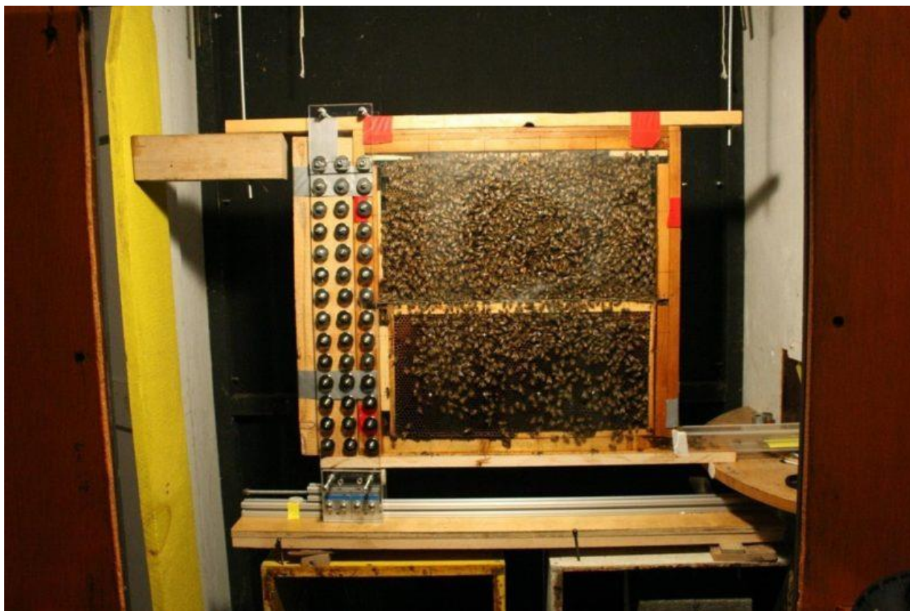
An observation bee hive fit with the magnetic insominator. Notice the plexiglass plates fitted with three columns of magnets on the left. These plates are moved from side to side to jostle test bees fitted with magnetic steel pieces but leave control bees fitted with non-magnetic copper pieces undisturbed. Photo: Barrett Klein
