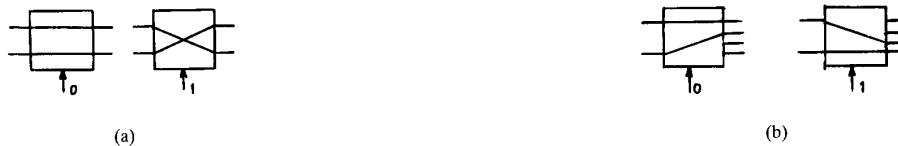
Fig. 6. Switching states of the SE's in the reconfigurable binary tree architecture: (a) SE in S_{k-1} to S_1 and (b) SE in S_0 .
