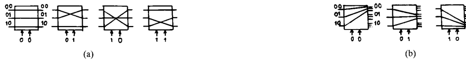
Fig. 11. Switching states of the SE's in the architecture with m = 3 : (a) SE in S_{k-1} to S_1 and (b) SE in S_0 .
