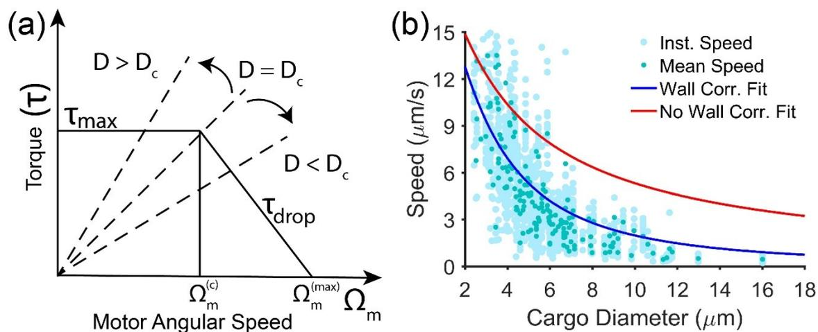
**Fig. S2:** (a) A schematic of the torque speed response curve of the bacterial motor. (b) Speed of oil-droplet loaded bacteria vs. cargo diameter. We have included the swimming speed of several smaller trajectories in addition to the longer trajectories presented in the manuscript.
