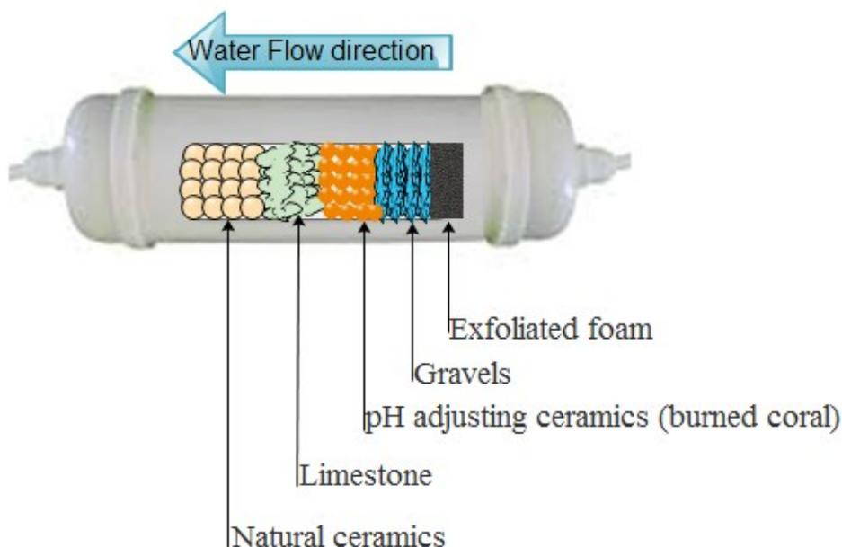
**Scheme-S 1:** Inline adsorption kit as designed for the experiments.
