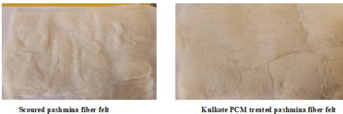
Figure 5: Scoured and Kulkote phase change material treated felt of pashmina fiber felt
