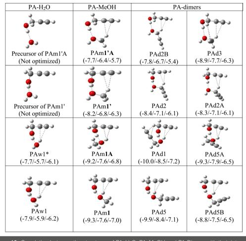
*Figure 16:* Correlation between the structures of PA–H<sub>2</sub>O, PA–MeOH and PA-Dimers with their interaction energies given as  $\Delta E_{\text{Raw}} / \Delta E_{\text{ZPC}} / \Delta E_{\text{BSSE}}$  in kcal/mol at the MP2/aug-cc-pVDZ level. (Reproduced from Ref. with permission from the Centre National de la Recherche Scientifique (CNRS) and The Royal Society of Chemistry).
