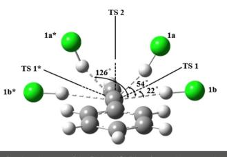
*Figure 14:* Depiction of various isomers of the PhAc–HCl (H– $\pi_{Ac}$ ) complexes together with the associated transition states, indicated by black solid lines. The angles indicate the orientation of the HCl internuclear axis with respect to the plane containing the phenyl ring. (Reproduced from Ref. with permission).
