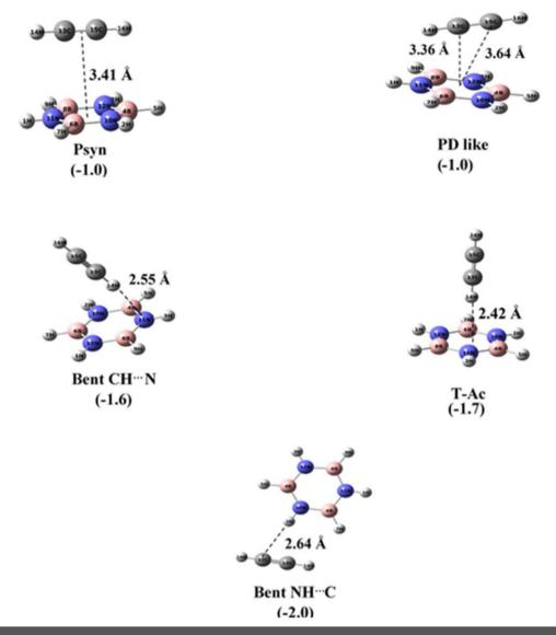
*Figure 10:* Optimized geometries of  $B_3N_3H_6-C_2H_2$  complexes at the MP2/aug-cc-pVDZ level of theory. BSSE corrected interaction energy, in kcal/mol, computed at the MP2/aug-cc-pVDZ level, is given in parenthesis, under each structure. (Reproduced from Ref.<sup>40</sup> with permission).
