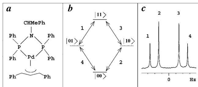
**Figure 6.** *a*, Organometallic compound (I) in which the two phosphorus ( $^{31}\text{P}$ ) nuclei constitute a two-spin-system. *b*, Energy level diagram of the two-spin-system. *c*, Equilibrium phosphorus spectrum recorded at 202 MHz in a magnetic field of 11.7 T.
