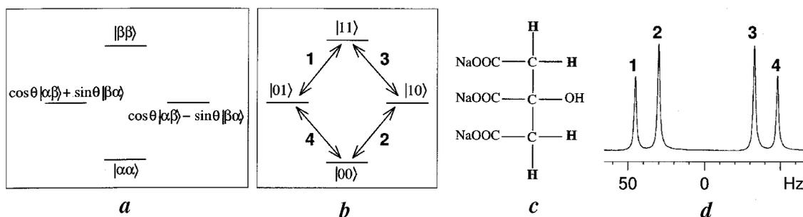
**Figure 1.** *a*, Eigenstates of a strongly coupled two-spin-system; *b*, Qubit labelling; *c*, Trisodium citrate yielding a strongly coupled two-spin-system, and *d*, Equilibrium 500 MHz  $^1\text{H}$  spectrum of *c*.
