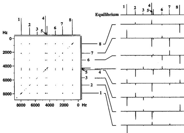
**Figure 9.** Z-COSY spectrum of oriented 3-bromo-1,2-dichlorobenzene. Equilibrium spectrum and cross-sections of the Z-COSY spectrum are shown on the right-hand-side.
