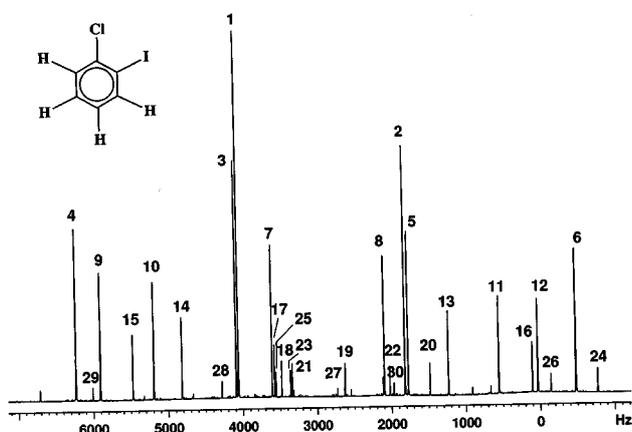
**Figure 14.** One-dimensional 500 MHz proton spectrum of 2-chloroiodobenzene oriented in liquid crystal ZLI-1132, at 300 K forming a four-qubit system. Transitions are labelled according to descending order of their intensities.
