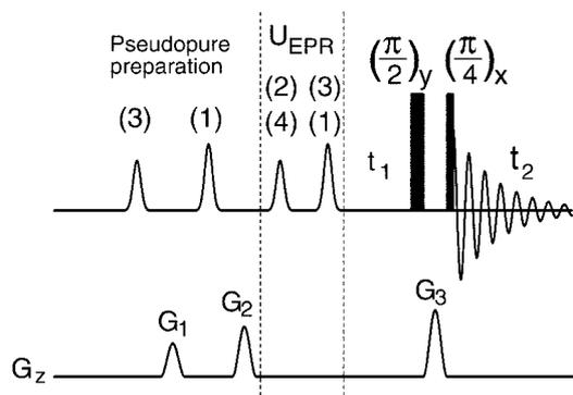
**Figure 5.** Pulse sequence for creation and tomography of EPR state. Numbers within parentheses indicate transition numbers as shown in Figure 1*d*.  $U_{\text{EPR}}$  is applied on transitions [(2), (3)] or [(4), (1)] as described in eq. (10) and Table 3.  $G_1$ ,  $G_2$  and  $G_3$  are field-gradient pulses of different strengths along the  $\hat{z}$ -direction.
