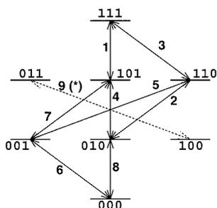
**Figure 10.** Energy level diagram of oriented 3-bromo-1,2-dichlorobenzene constructed using the Z-COSY spectrum shown in Figure 9. Transitions are labelled as in Figure 8. Only nine transitions are assigned. The remaining transitions have very low intensity.
