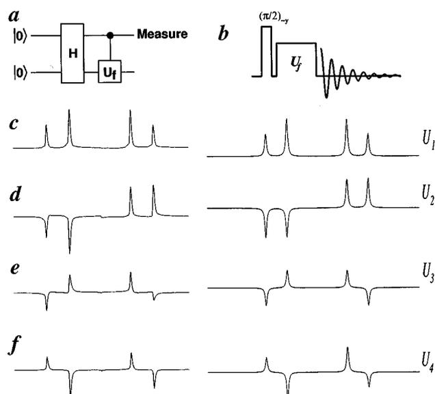
**Figure 3.** Implementation of DJ algorithm. *a*, Quantum circuit. *b*, Experimental scheme for the implementation of DJ algorithm. *c, d*, Experimental spectra corresponding to the two constant functions of  $U_1$  and  $U_2$  respectively. *e, f*, Spectra corresponding to the two balanced functions of  $U_3$  and  $U_4$  respectively. Expected spectra for all the four functions are given on the right-hand-side.
