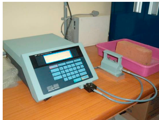
Fig. 2. Quick Thermal Conductivity Meter (QTM-500) for measuring thermal conductivity.
