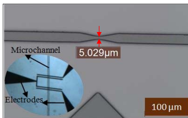
Figure 3: 5 \mu\text{m} constriction in the microchannel, post SU8 lithography; Inset: Gold electrodes integrated with the PDMS microchannel
