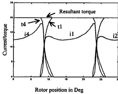
Fig. 7 Computed currents and the torque using Method 4 at 150 rpm for a bus voltage of 560V
