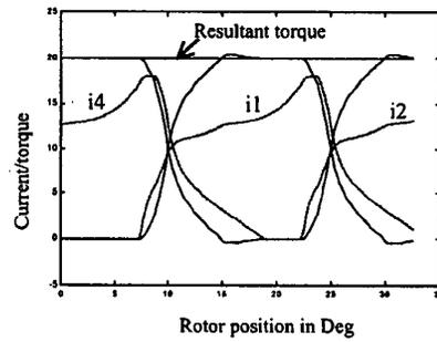
Fig. 7 Computed currents and the torque using Method 4 at 450 rpm for a bus voltage of 560V
