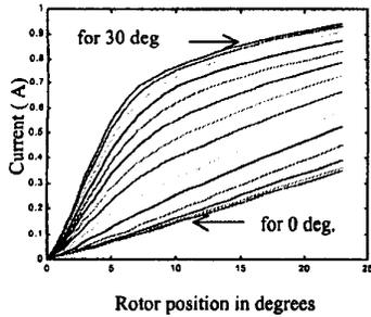
Fig 1. Flux-linkage characteristics of 4 kW SRM
