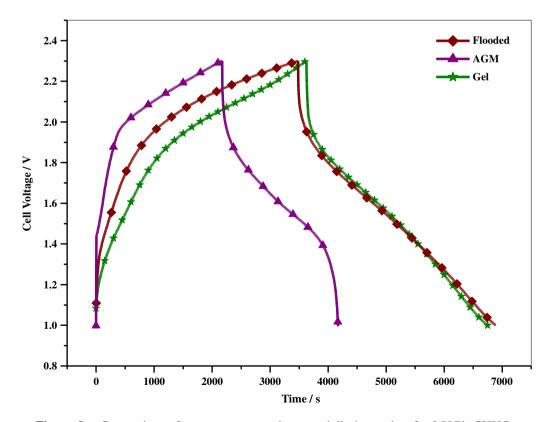
Figure 9. Comparison of constant-current charge and discharge data for 2 V Pb-CHUCs.
