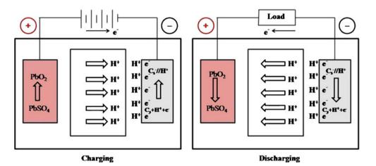
Figure 1. Charge-discharge schematic of a hybrid ultracapacitor.
