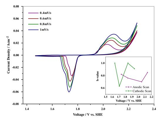
**Figure 7.** Cyclic voltammograms for substrate-integrated  $PbO_2$  electrode at varying scan rates. Inset: calculated b-values for a substrate-integrated  $PbO_2$  electrode as a function of potential for the anodic and cathodic sweep.
