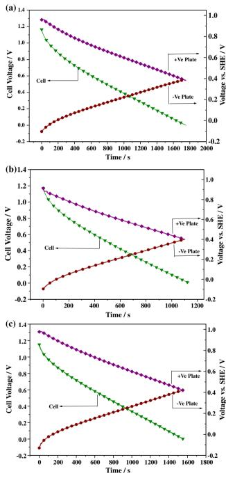
**Figure 5.** Constant-current discharge cures for symmetric carbon cell and single electrodes in (**a**) flooded, (**b**) AGM and (**c**) gel systems.
