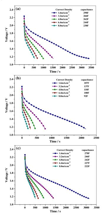
**Figure 10.** Constant current discharge data for 2 V Pb-C HUC at varying discharge current-loads for (**a**) flooded, (**b**) AGM, and (**c**) gel HUCs.
