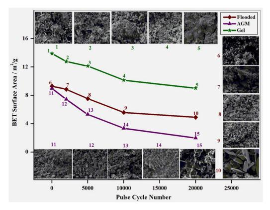
Figure 11. Effect of pulsed charge and discharge cycling on the surface area of SI–PbO<sub>2</sub> during cycling.
