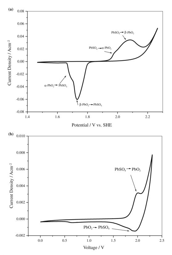
Figure 6. Cyclic voltammograms for (a) substrate-integrated lead electrode and (b) hybrid ultracapacitor single cell.
