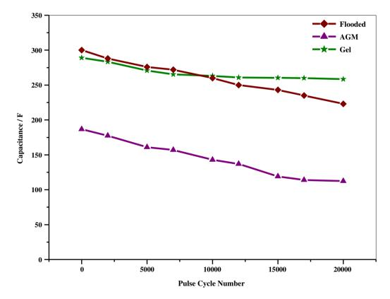
Figure 12. Effect of pulsed charge and discharge cycling on the capacitance for HUCs.
