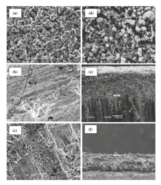
**Figure 3.** SEM images for (**a**) high surface-area-carbon, (**b**) lead sheet, (**c**) lead sheet after etching with nitric acid, (**d**) substrate-integrated PbO<sub>2</sub>, (**e**) cross-sectional view of substrate-integrated PbO<sub>2</sub> electrode, and (**f**) cross-sectional view of carbon coated graphite electrode. Scale bar: (**a**) 10  $\mu$ m; (**b**) 10  $\mu$ m; (**c**) 5  $\mu$ m; (**d**) 10  $\mu$ m; (**e**) 50  $\mu$ m; (**f**) 100  $\mu$ m.
