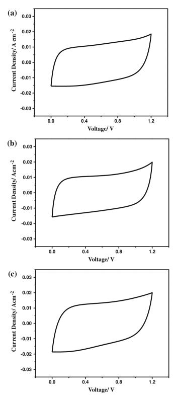
**Figure 4.** Cyclic voltammograms for MWV X-090177 carbon electrodes at scan rate of 10 mV/s in (**a**) flooded, (**b**) AGM and (**c**) gel electrolytes.
