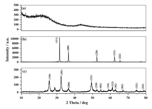
Figure 2. XRD patterns for (a) high surface-area-carbon, (b) pure lead-sheet, and (c) substrate-integrated lead dioxide.
