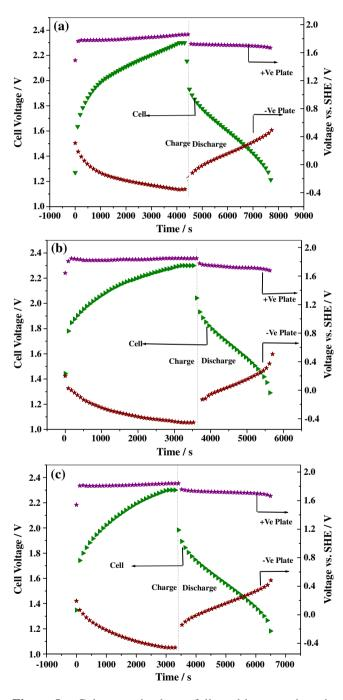
**Figure 8.** Galvanostatic charge followed by potentiostatic charge and galvanostatic discharge for 2 V Pb-C HUCs with single electrode charge-discharge profiles for (**a**) flooded, (**b**) AGM, (**c**) gel configurations.
