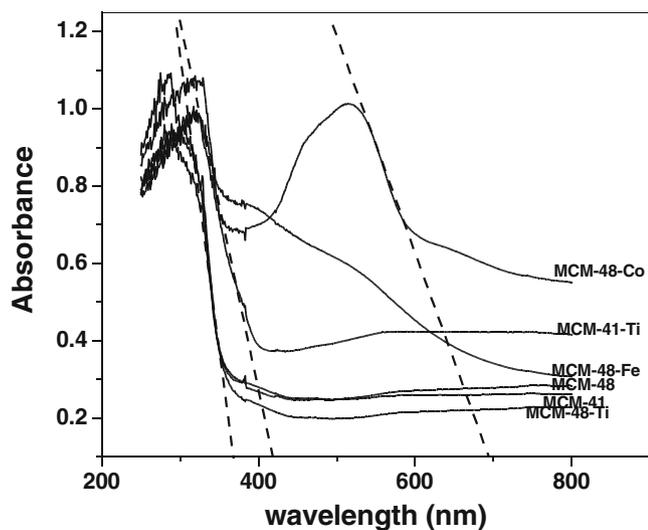
**Figure 4.** UV-vis spectra of the various catalysts.
