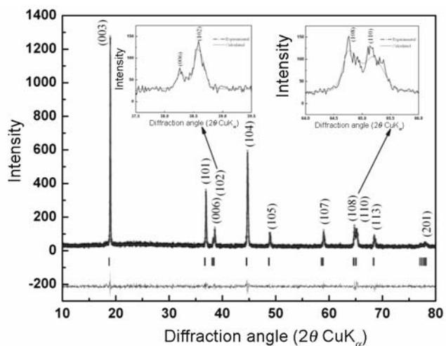
**Figure 1.** Powder XRD Rietveld fit for  $\text{LiNi}_{0.8}\text{Co}_{0.2}\text{O}_2$  derived from nitrates-melt decomposition.
