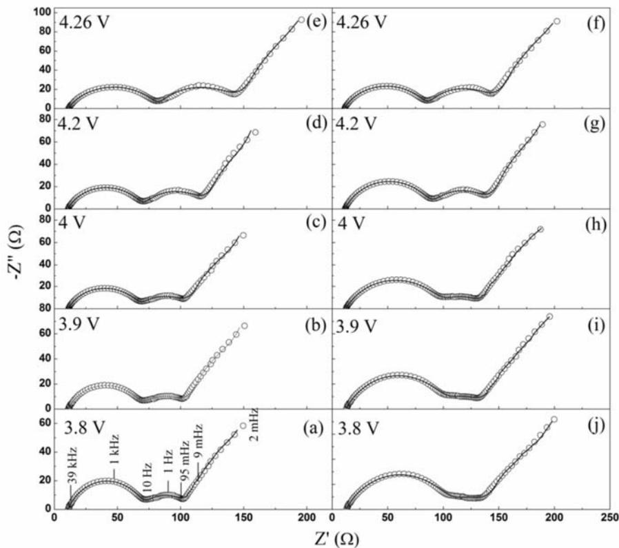
**Figure 6.** Nyquist plots for  $\text{LiNi}_{0.8}\text{Co}_{0.2}\text{O}_2$  half cells during de-intercalation (a–e) and intercalation (f–j) of lithium.
