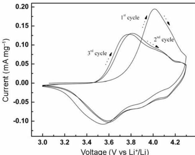
**Figure 3.** Cyclic voltammograms for  $\text{LiNi}_{0.8}\text{Co}_{0.2}\text{O}_2$  vs  $\text{Li}$  cells in voltage range 3–4.3 V with a scan rate of 0.1 mV/s.
