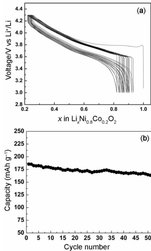
**Figure 4.** (a) Voltage vs composition data derived from galvanostatic charge/discharge experiments on  $\text{LiNi}_{0.8}\text{Co}_{0.2}\text{O}_2/\text{Li}$  cell in voltage range between 3 and 4.3 V at 0.2C rate and (b) discharge capacity vs cycle number.
