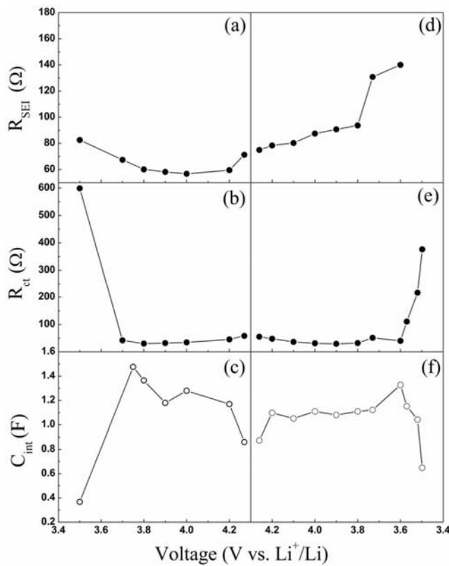
**Figure 8.** Variation in resistive and capacitive components for cell during lithium de-intercalation (a–c) and intercalation (d–f). Resistance due to SEI layer is denoted as  $R_{SEI}$  (a, d) and charge transfer resistance as  $R_{ct}$  (b, e).
