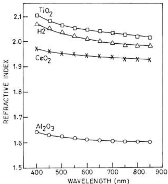
**Figure 3.** Optical dispersion characteristics of single layer thin films as described in figure 2.
