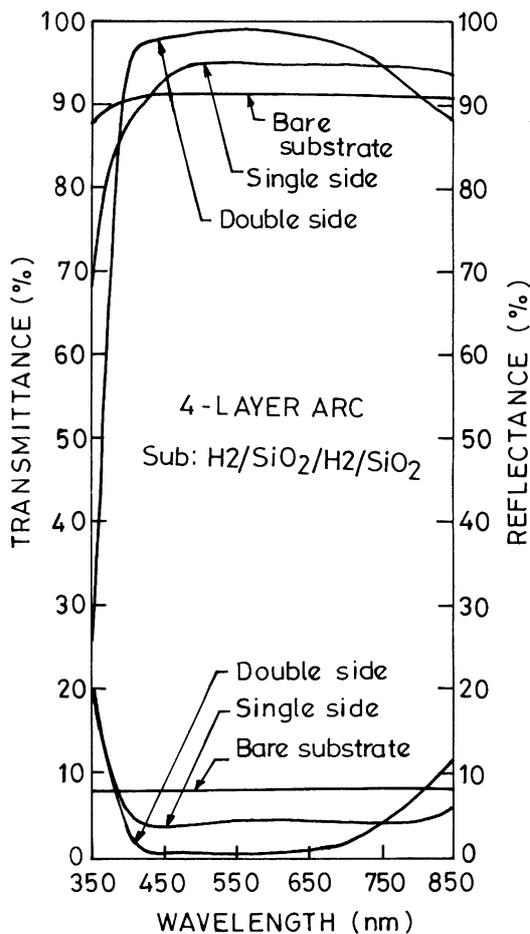
Figure 7. Measured spectral characteristics of 4-layer antireflection coatings deposited on glass.
