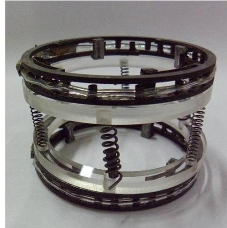
Fig. 17: Completed prototype with two clamping rings, linearly-actuating SMA springs, and bias springs. The SMA springs are shown extended.
