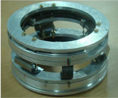
Fig. 2: The prototype of the crawling device. It is bulky because of its housing for the clamping rings and is slow because of the SMA strips that take a long time to heat and cool, especially to cool.
