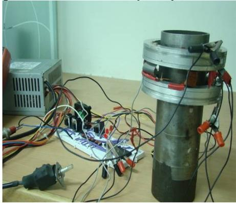
Fig. 3: Test set-up of the crawling device with clamping rings, SMA strip for linear actuation and control circuit to effect cyclical triggering of the three actuators, namely, two SMA wires and one set of SMA strips.
