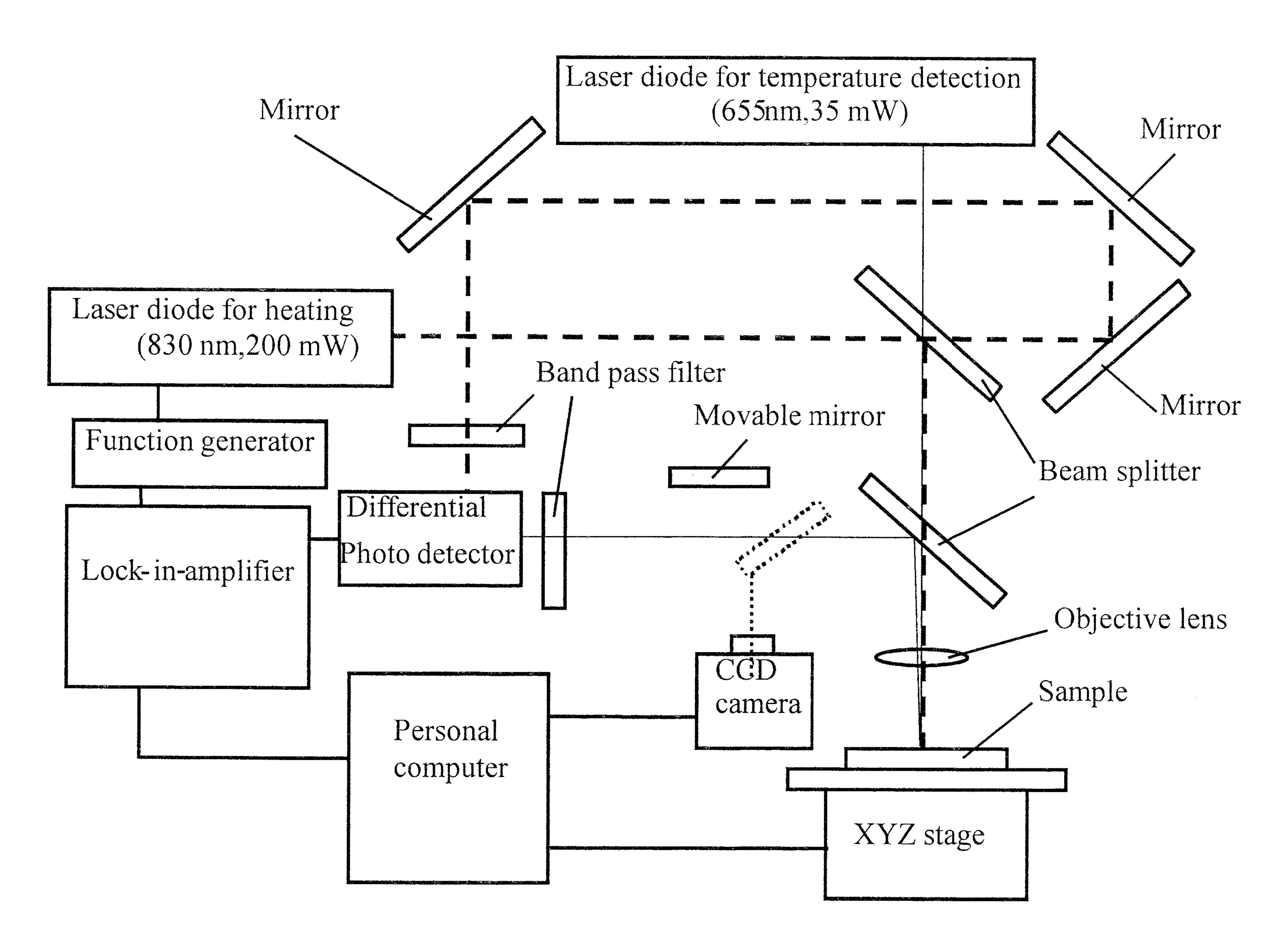
Fig. 2: Schematic diagram of the thermal microscope used in this study.
