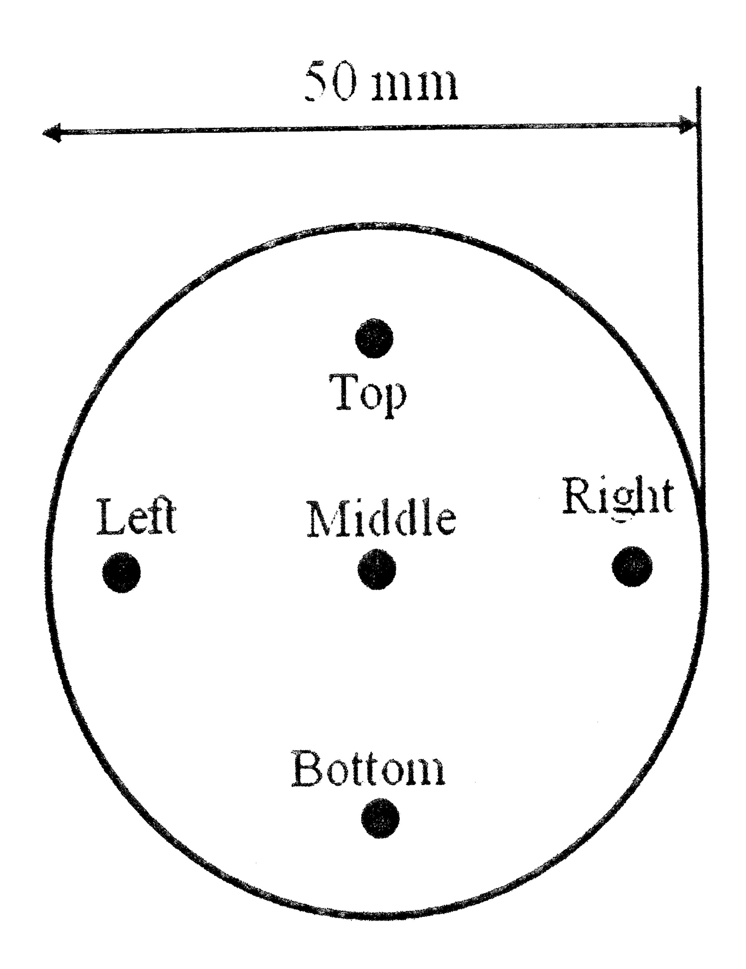
Fig. 1: Locations on the surface of  $Al_xGa_{l-x}N$  sample used for measurements.
