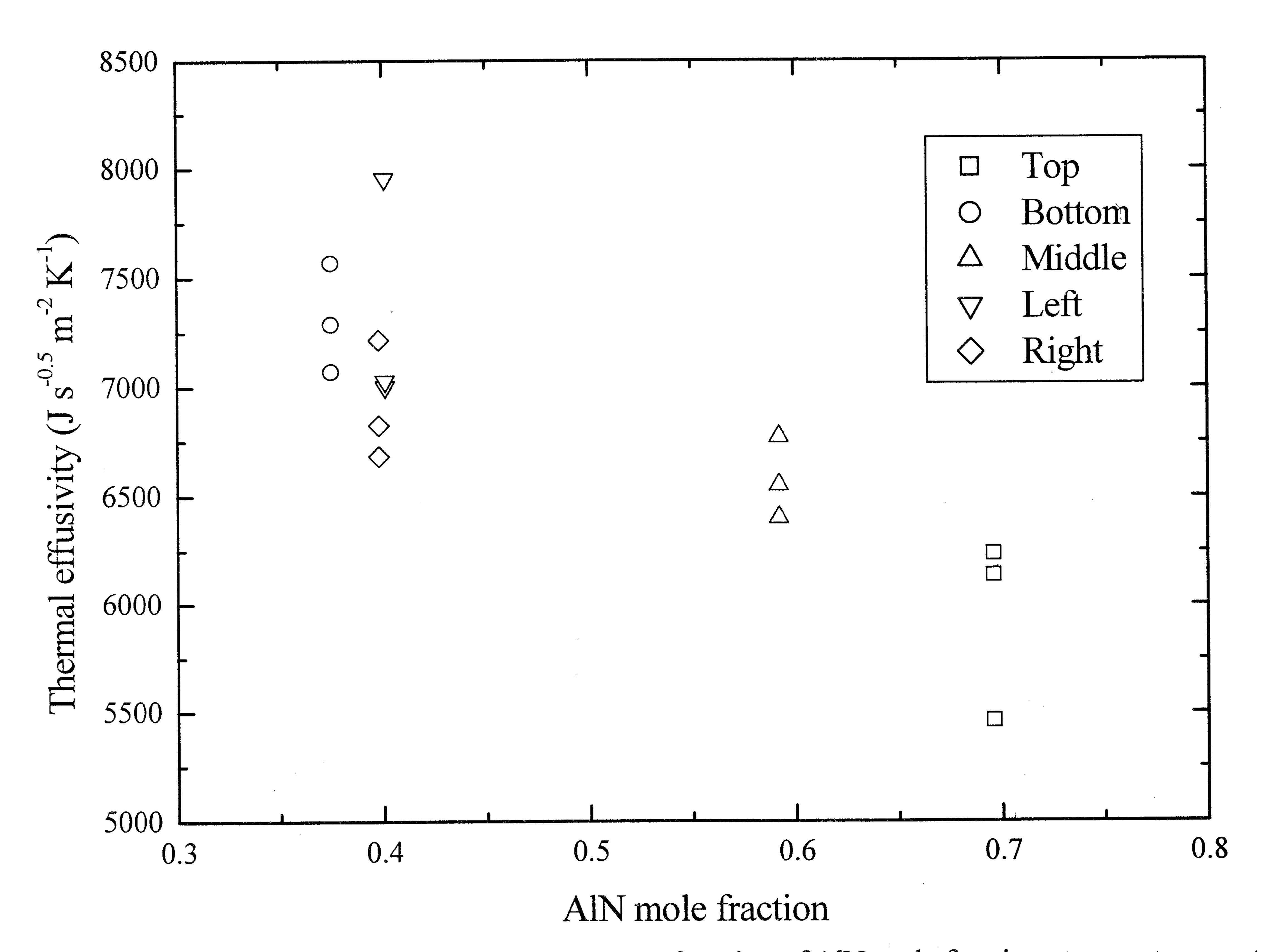
Fig. 3: Measured thermal effusivity of  $Al_xGa_{l-x}N$  as a function of AlN mole fraction at room temperature.
