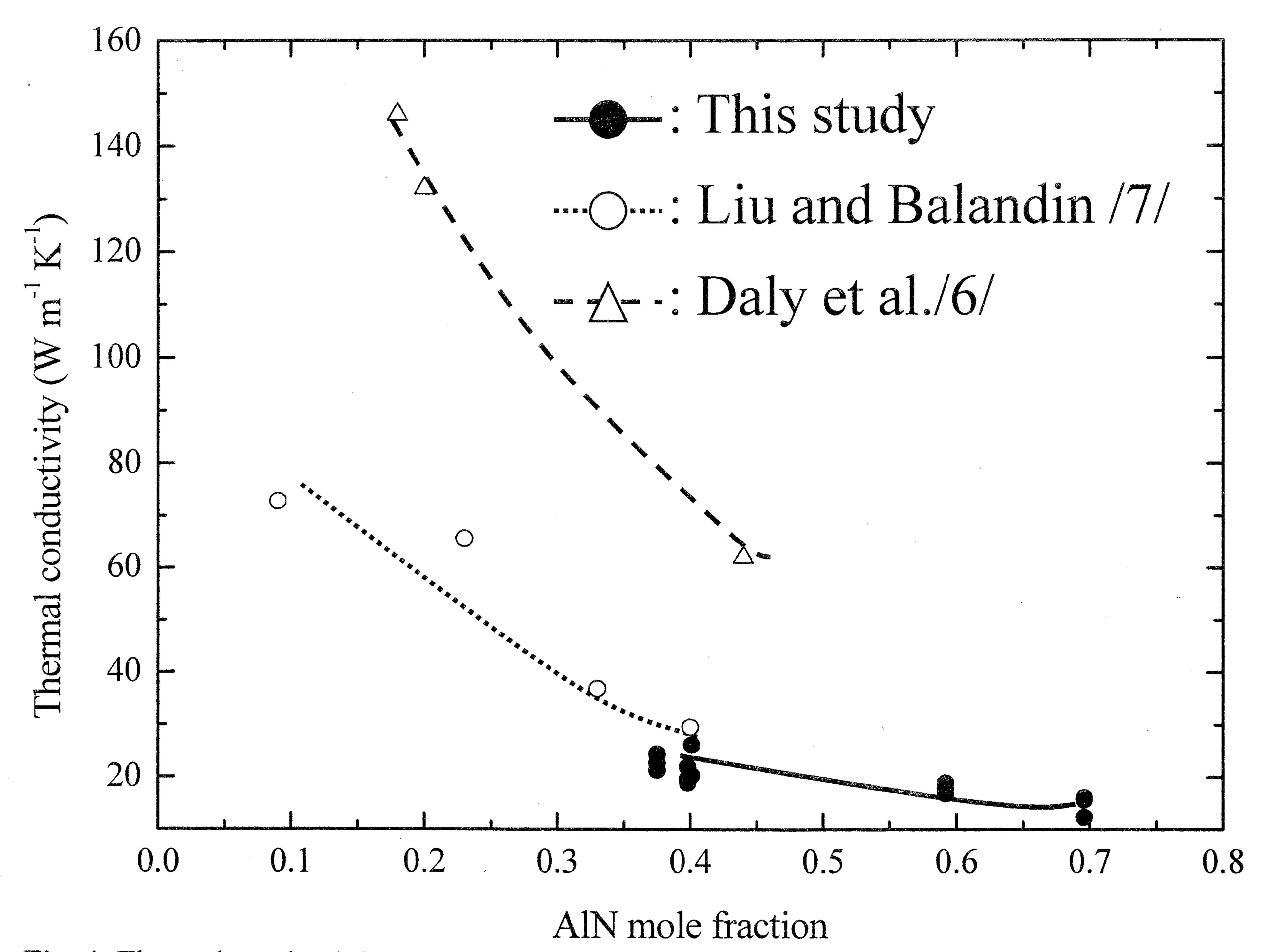
Fig. 4: Thermal conductivity of  $Al_xGa_{l-x}N$  as a function of AlN mole fraction at room temperature.
