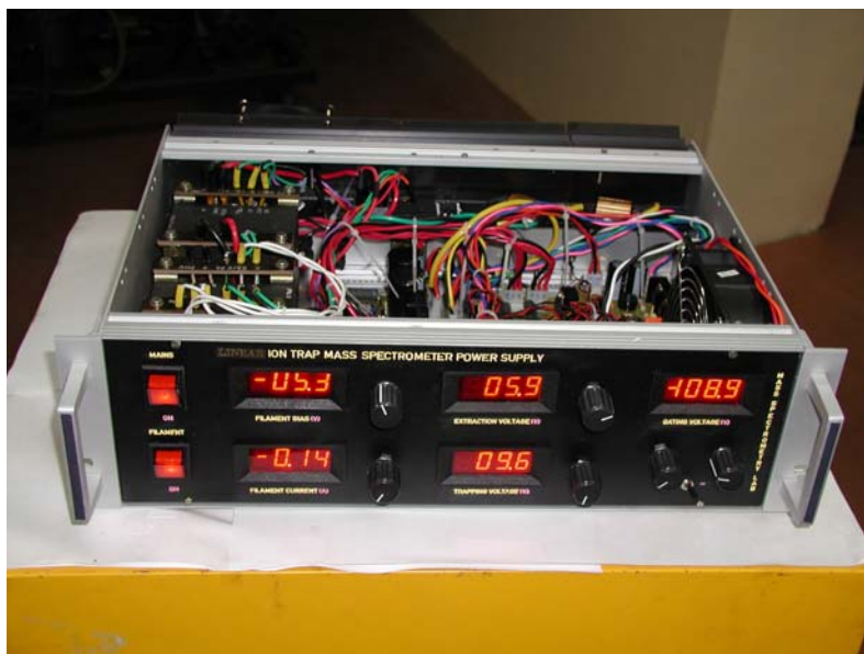
Fig. 8. Power supply unit for linear ion trap mass spectrometer
