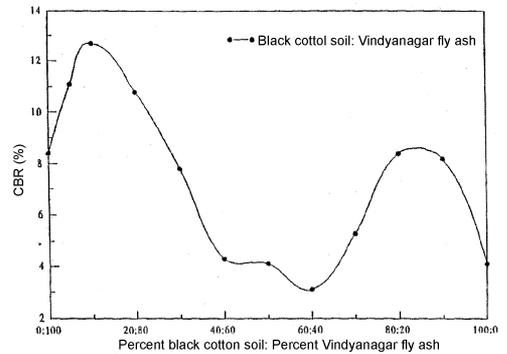
FIG. 10. CBR values of black cotton soil–Vindyanagar fly ash mixtures.
