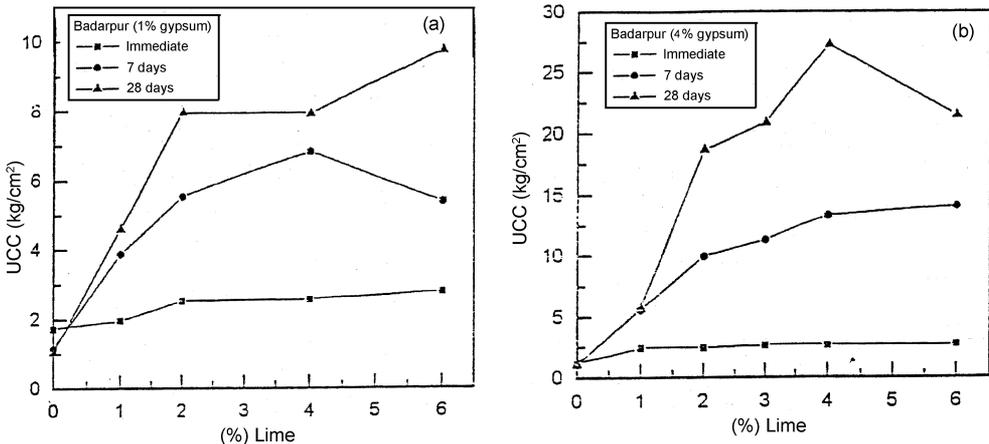
FIG. 8. Effect of lime and curing on the UCC of (a) Badarpur fly ash + 1% gypsum, and (b) Badarpur fly ash + 4% gypsum.
