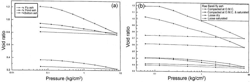
FIG. 12. Void ratio–pressure relationship for Rae Bareli (a) coal, and (b) fly ashes at different placement conditions.
