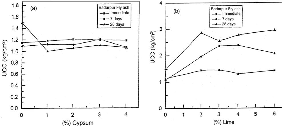
FIG. 7. Effect of (a) gypsum and curing, and (b) lime and curing on the unconfined compressive (UCC) strength of Badarpur fly ash.
