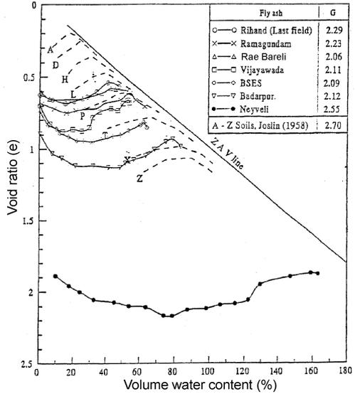
FIG. 3. Void ratio vs volume water content relation for fly ashes and soils.
