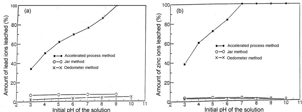
FIG. 15. Comparison of leaching of (a) lead, and (b) zinc ions by three methods for fly ash (N).
