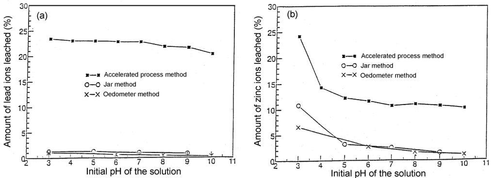
FIG. 16. Comparison of leaching of (a) lead, and (b) zinc ions by three methods for fly ash (B).
