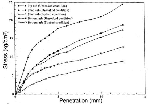
FIG. 9. Stress vs penetration of Badarpur coal ashes.
