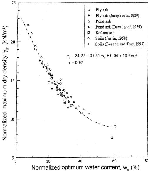
FIG. 6. Maximum dry density vs optimum water content based on normalized parameters for coal ashes and soils.
