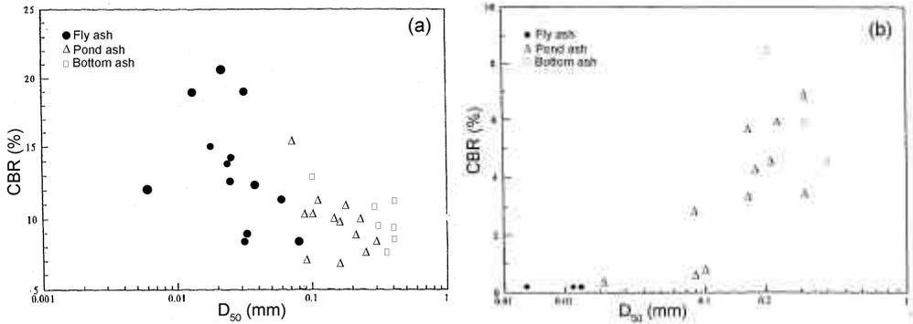
FIG. 11. CBR values vs  $D_{50}$  for (a) unsoaked, and (b) soaked conditions.
