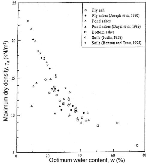
FIG. 5. Maximum dry density vs optimum water content for coal ashes and soils.
