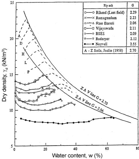
FIG. 2. Dry density vs water content relation for fly ashes and soils.
