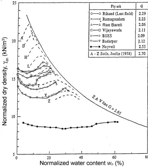
FIG. 4. Normalized dry density vs normalized water content for fly ashes and soils.
