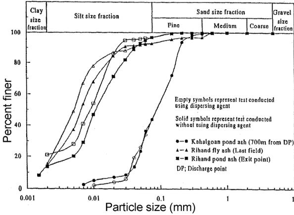
FIG. 13. Effect of dispersing agent on the particle size distribution of coal ashes.
