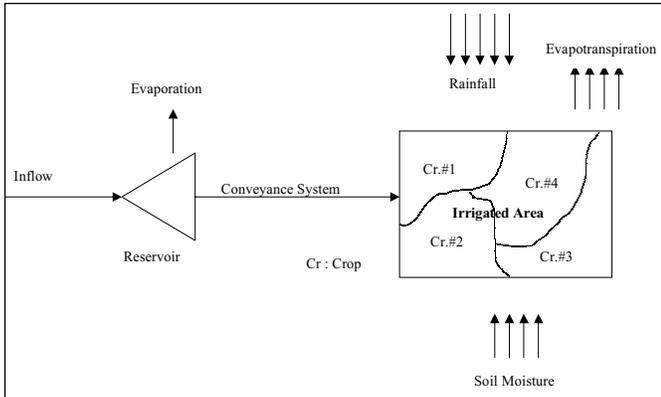
Figure 2. Components of a Typical Surface Water Irrigation System.
