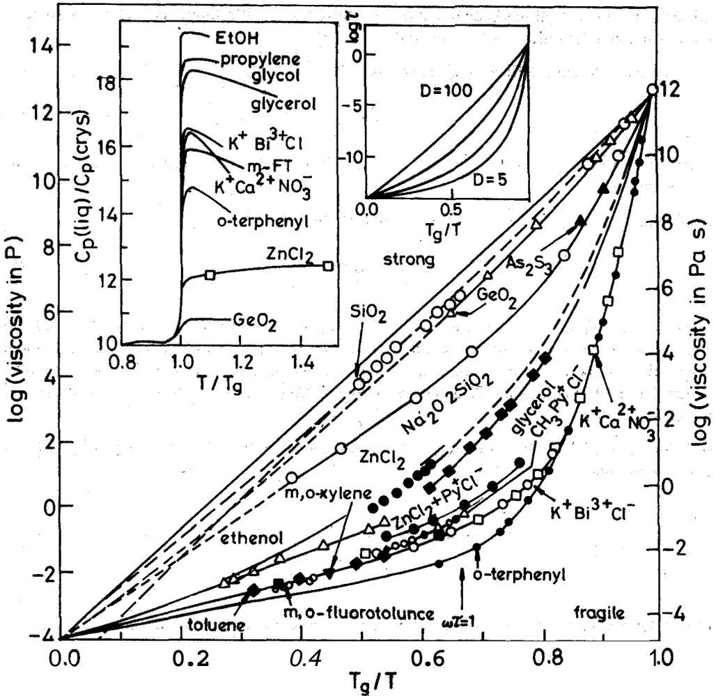
Fig. 6. Plot of  $\log$  viscosity as a function of scaled temperature (from Angell<sup>3</sup>).
