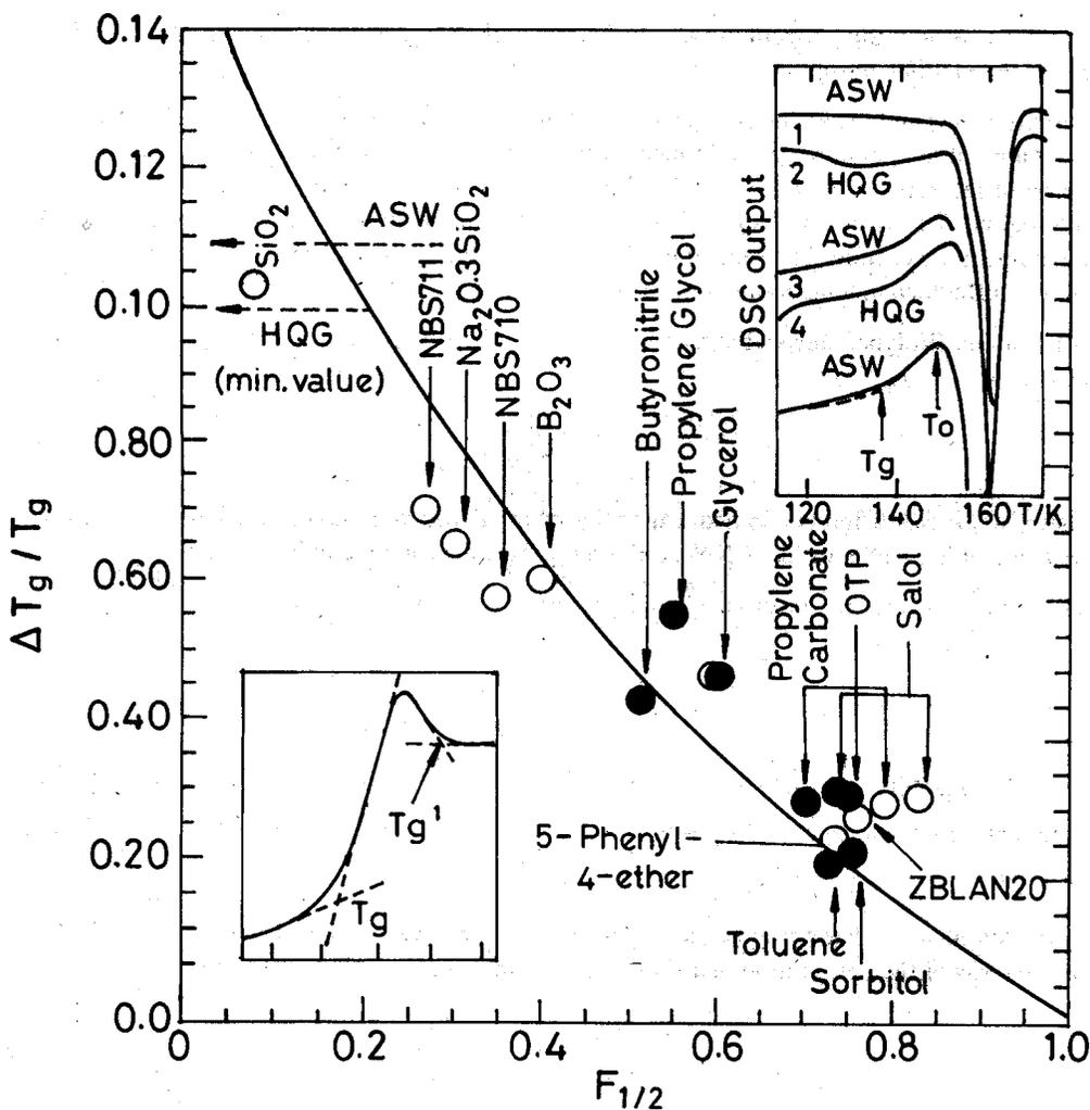
FIG. 7.  $\text{IMA}^{12}$  plot  $\Delta T_g / T_g$  vs  $F_{1/2}^{\text{Relx}}$ . The smooth line is function in eqn (12).
