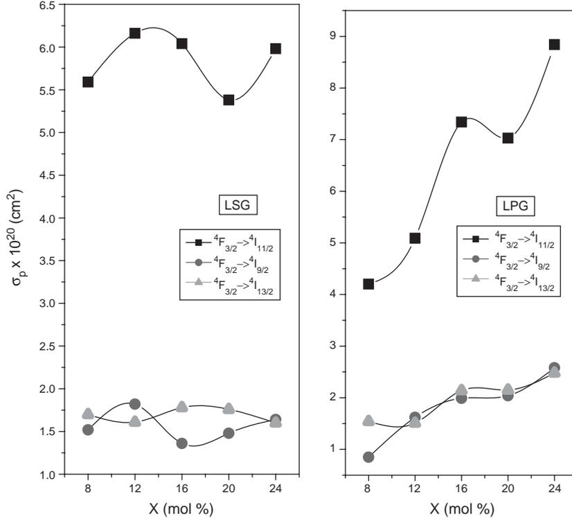
Fig. 6. Variation of emission cross-section ( $\sigma_p$ ) with  $x$  in lithium sodium (LSG) and lithium potassium (LPG) mixed alkali borate glasses.
