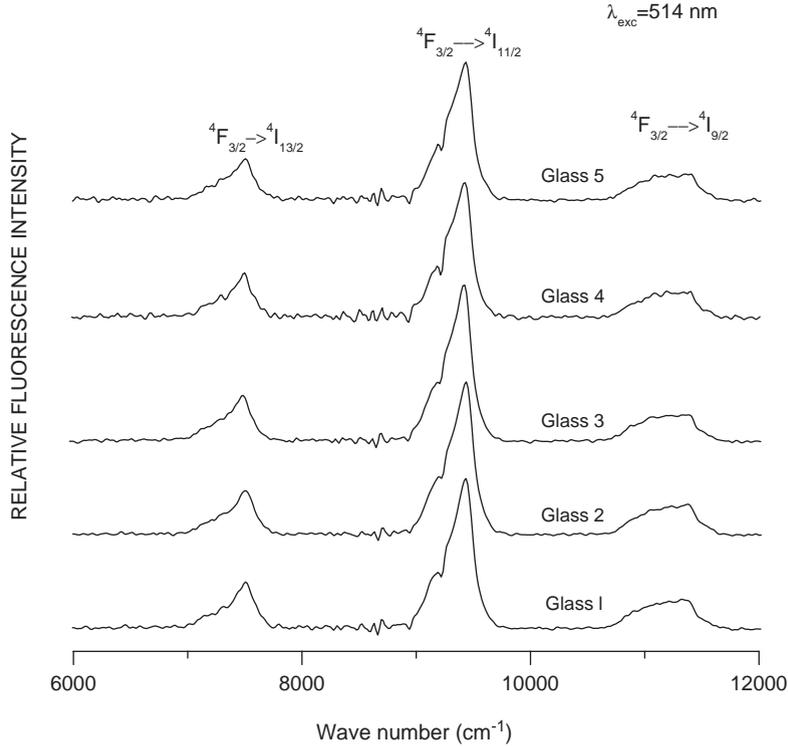
Fig. 5. Luminescence spectra of  $\text{Nd}^{3+}$  in  $67\text{B}_2\text{O}_3 \cdot x\text{Li}_2\text{O} \cdot (32-x)\text{Na}_2\text{O}$  ( $x = 8, 12, 16, 20$  and  $24$ ) glasses.
