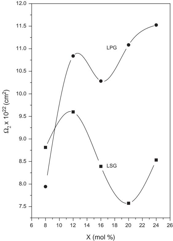
Fig. 2. Variation of  $\Omega_2$  ( $\times 10^{20}$ ) with  $x$  in lithium sodium (LSG) and lithium potassium (LPG) mixed alkali borate glasses.
