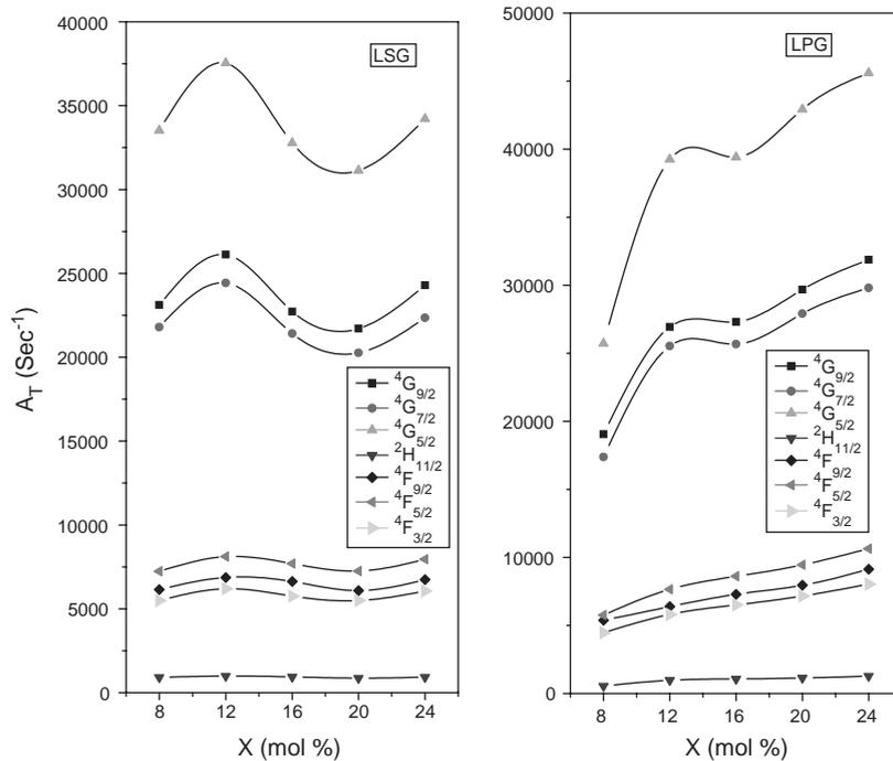
Fig. 4. Variation of total radiative transition probabilities ( $A_T$ ) with  $x$  in lithium sodium (LSG) and lithium potassium (LPG) mixed alkali borate glasses.
