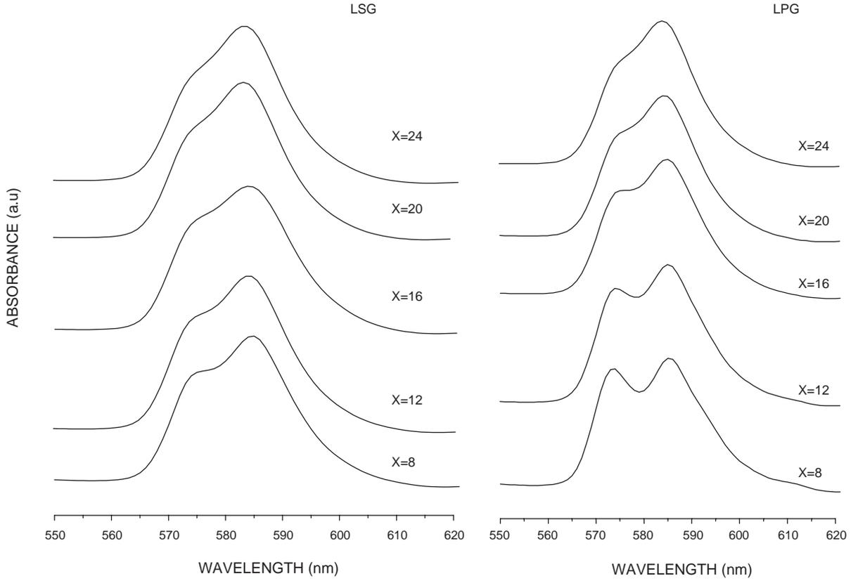
Fig. 3. Variation of spectral profiles of hypersensitive transition  ${}^4F_{3/2} \rightarrow {}^4G_{5/2} + {}^2G_{7/2}$  with  $x$  in lithium sodium (LSG) and lithium potassium (LPG) mixed alkali borate glasses.
