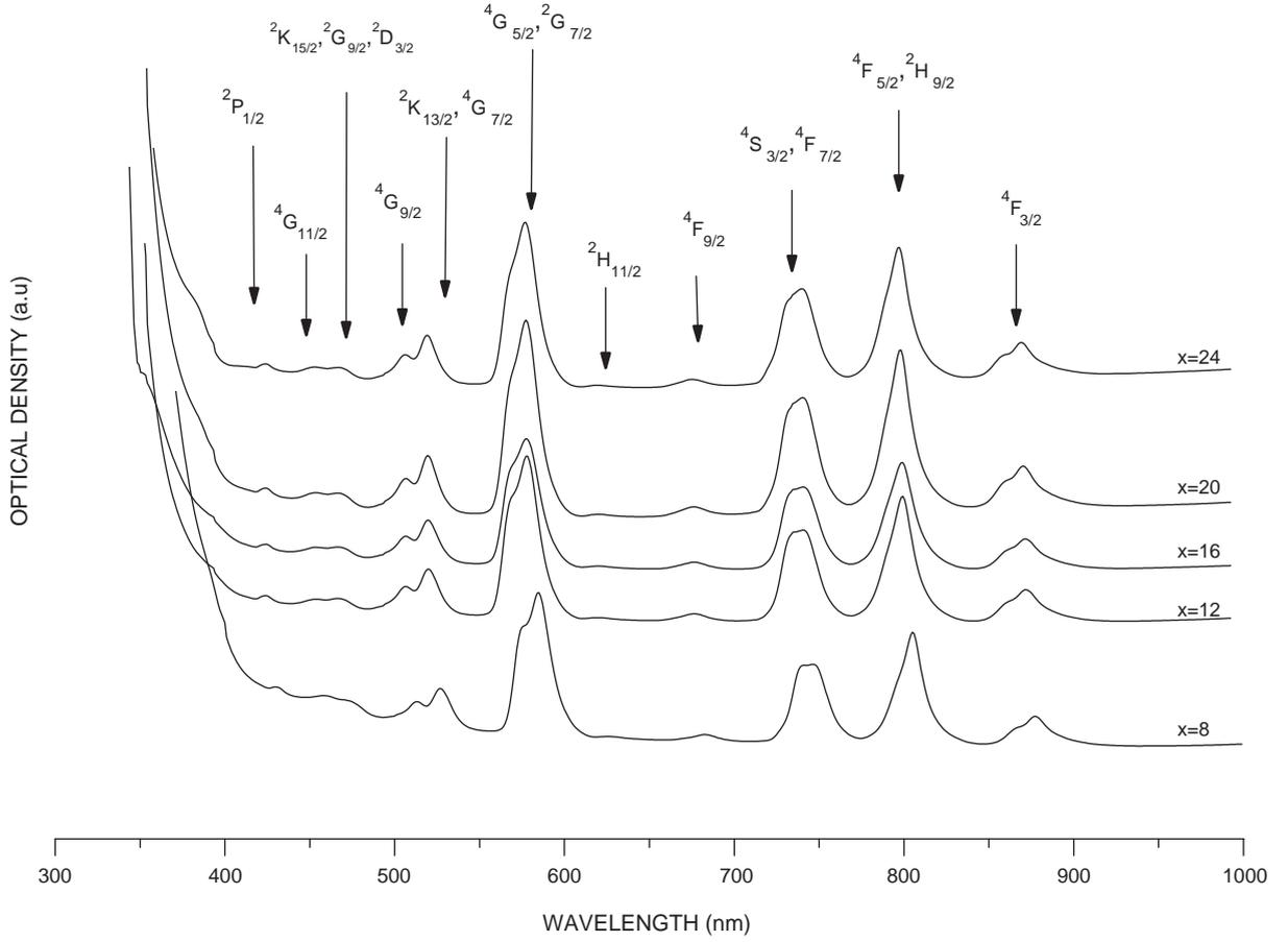
Fig. 1. Optical absorption spectra of  $\text{Nd}^{3+}$  doped  $67\text{B}_2\text{O}_3 \cdot x\text{Li}_2\text{O} \cdot (32-x)\text{Na}_2\text{O}$  ( $x=8, 12, 16, 20$  and  $24$ ) glasses
