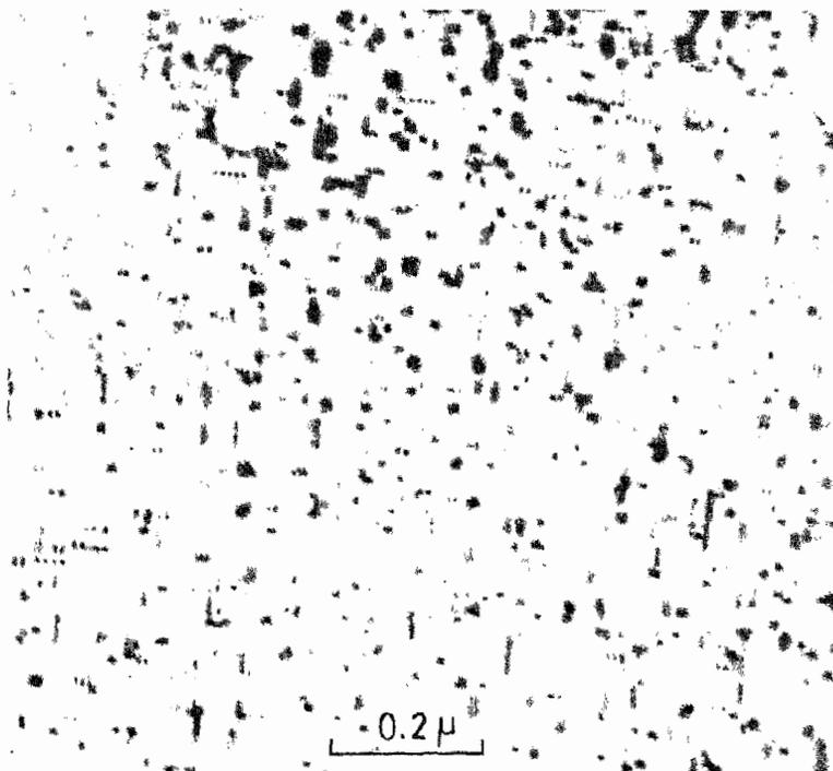
Figure 2. Electron micrograph of partially-aged sample showing small and dense rod-shaped precipitates ( $T_s = 450^\circ\text{C}$ ,  $T_a = 165^\circ\text{C}$ ,  $t_a = 18$  hr).
