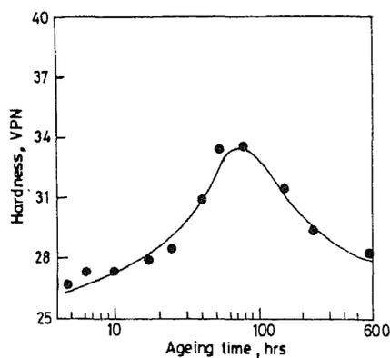
Figure 1. Hardness variation with time during ageing at  $165^\circ\text{C}$  ( $T_d = 450^\circ\text{C}$ ).
