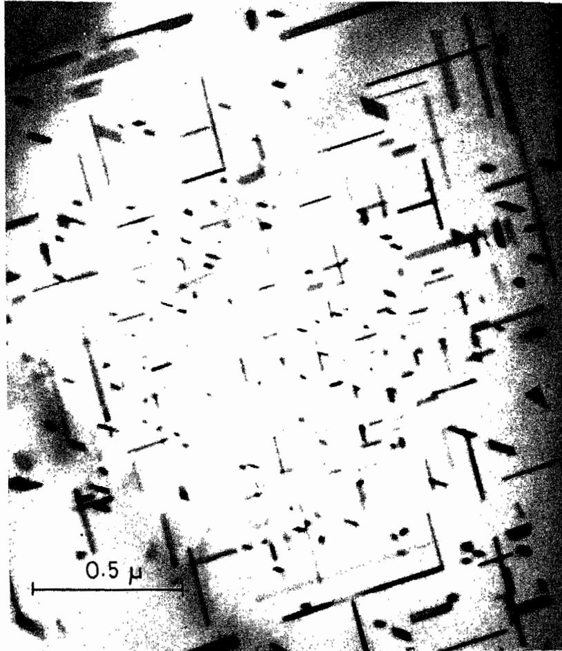
**Figure 3.** A TEM photograph of the peak-hardened alloy (70 hr at 165°C) showing rod-, triangular-, and rectangular-shaped precipitates.
