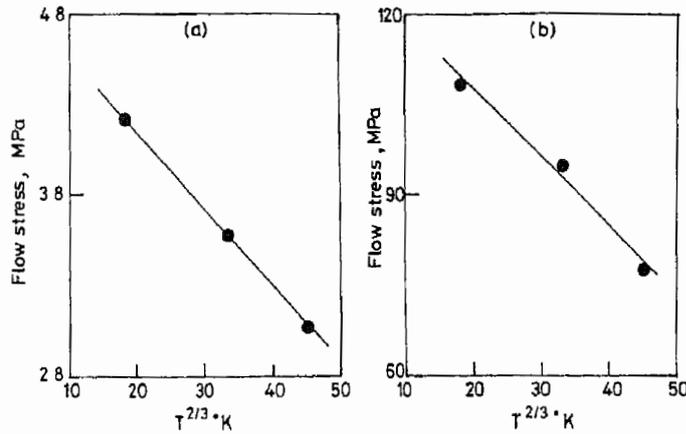
Figure 5. Flow stress-(temperature)<sup>2/3</sup> relation for (a), under-aged (b), peak-aged conditions ( $\dot{\epsilon} = 9.8 \times 10^{-4} \text{ sec}^{-1}$ ).
