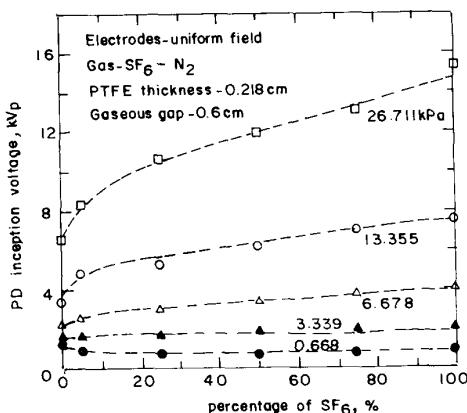
Figure 5 - Measured PD inception voltages in SF<sub>6</sub>-N<sub>2</sub>-PTFE composite dielectric at different percentages of SF<sub>6</sub> for a 0.6 cm gaseous gap.
