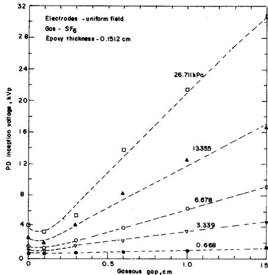
Figure 3 - Measured PD inception voltages in SF<sub>6</sub>-Epoxy composite dielectric.
