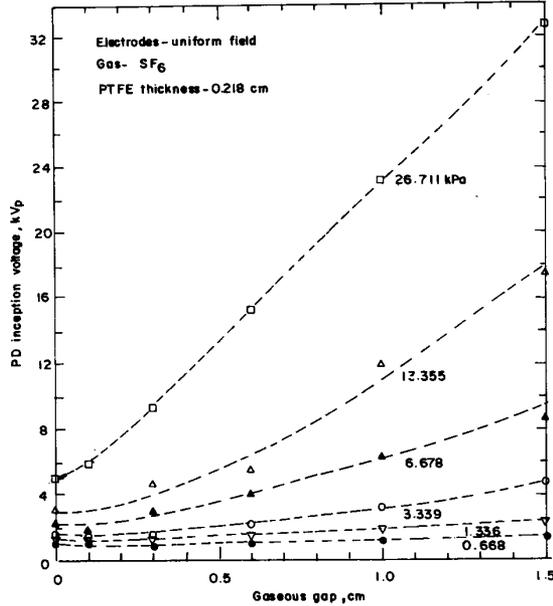
Figure 2 - Measured PD inception voltages in SF<sub>6</sub>-PTFE composite dielectric.
