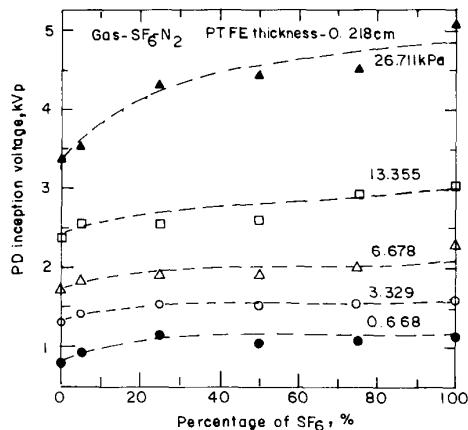
Figure 4 - Measured PD inception voltages in SF<sub>6</sub>-N<sub>2</sub>-PTFE composite dielectric at different percentages of SF<sub>6</sub> in case of surface discharges (0.0 cm gaseous gap).
