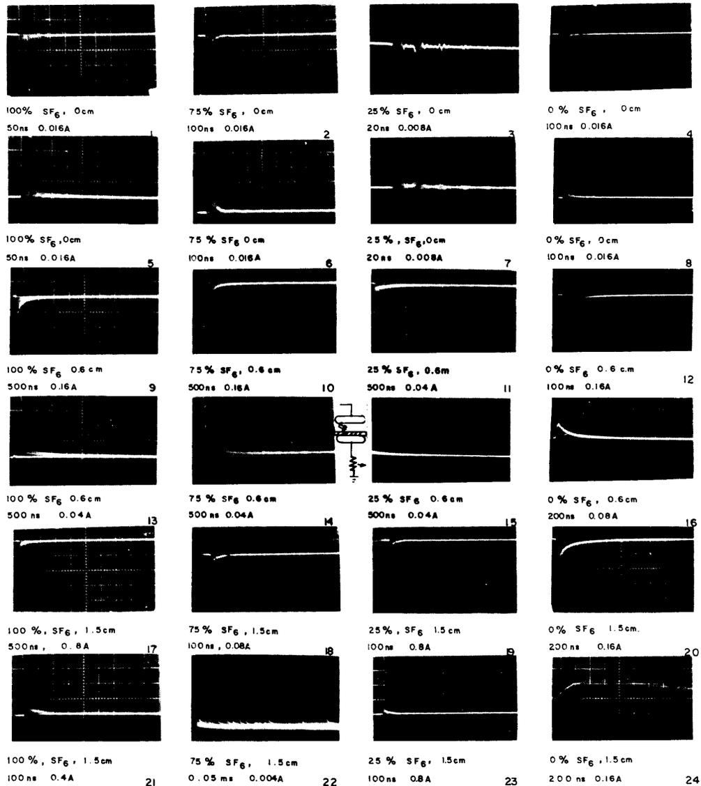
Figure 7 - Pd pulses in SF<sub>6</sub>-N<sub>2</sub>-PTFE combination at 26.71 kPa at different percentages of SF<sub>6</sub> and at different gaseous gaps. (Scale divisions are given by indicated times and currents).
