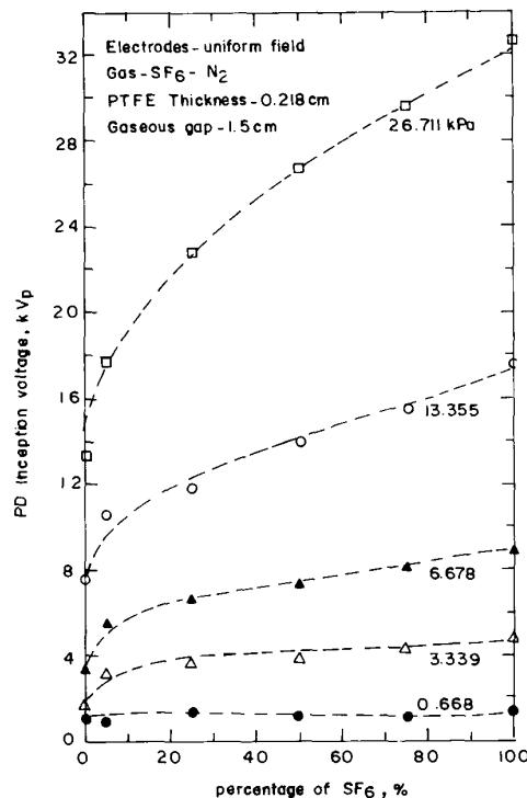
Figure 6 - Measured PD inception voltages in SF<sub>6</sub>-N<sub>2</sub>-PTFE composite dielectric at different percentages of SF<sub>6</sub> for a 1.5 cm gaseous gap.
