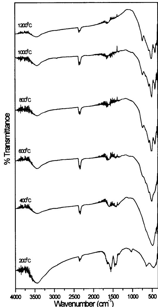
**Figure 2.** Infrared spectroscopy of the zirconia samples heated to various temperatures.
