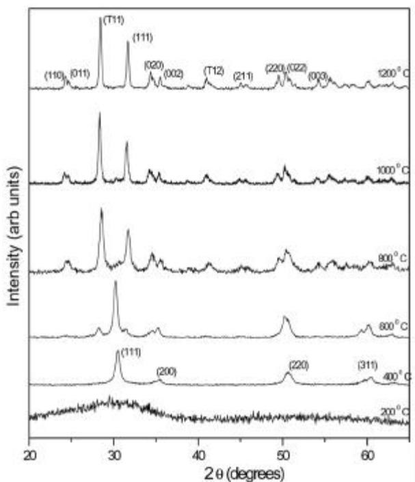
**Figure 1.** Evolution of the X-ray diffraction pattern with heat treatment at elevated temperatures for the case of Al<sub>2</sub>O<sub>3</sub>.
